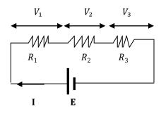
Since by Ohms law, V = IRand  $E = V_1 + V_2 + V_3 - 1$ , where  $E = IR_S$   $\Rightarrow V_1 = IR_1, V_2 = IR_2$  and  $V_3 = IR_3$ now substituting in 1<sup>st</sup> we have  $IR_s = IR_1 + IR_2 + IR_3$   $\Rightarrow I(R_S) = I(R_1 + R_2 + R_3)$  $\Rightarrow R_S = (R_1 + R_2 + R_3)$  Resistance in parallel combination: -
