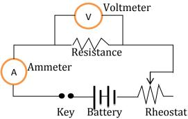
First we close the key so that current flows in the circuit and after that adjust the rheostat so that minimum current flows in the circuit.
