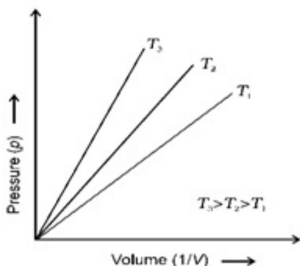
Ans. It represents the graph between p and 1/V. It is a straight line passing through origin. However at high pressures, gases deviate from Boyle's law and under such conditions a straight line is not obtained in the graph.
