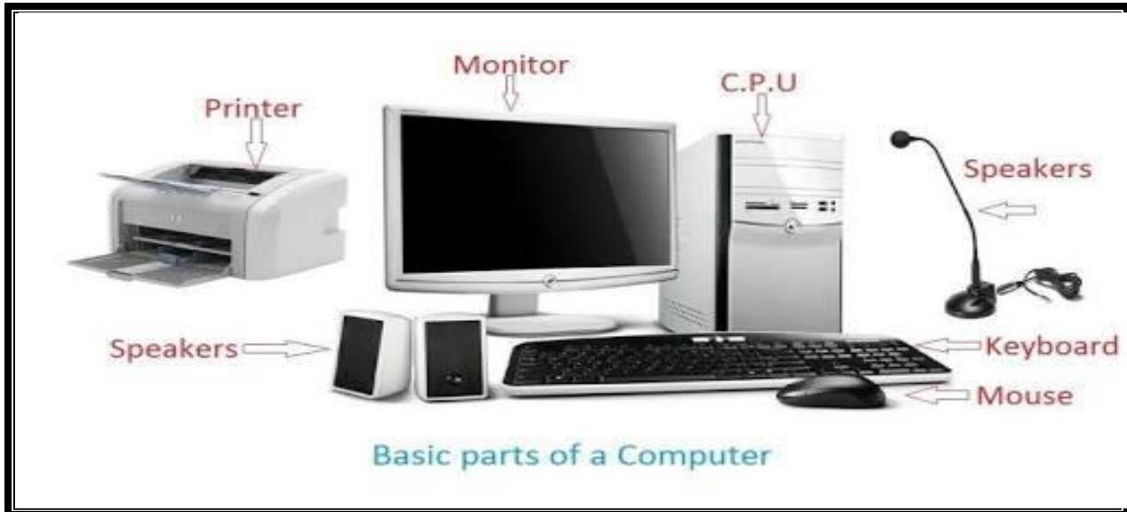
**A computer has four main parts , which help in performing the IPO cycle.**
