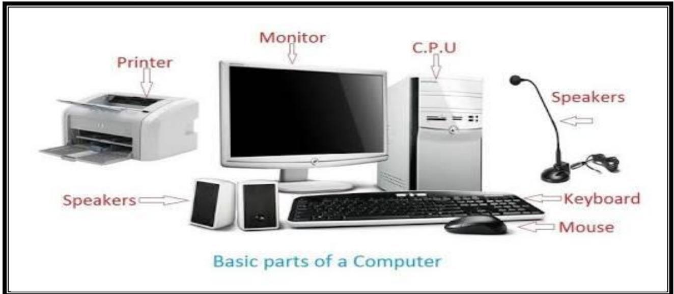
**A computer has four main parts , which help in performing the IPO cycle.**
